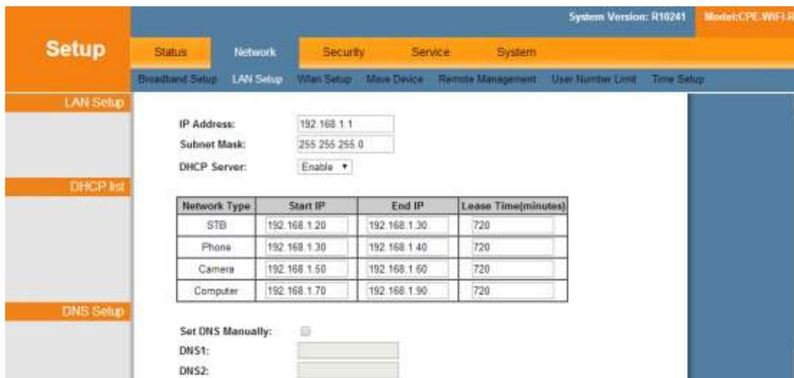
1. DHCP Enable: You can select the "Enable / Disable" DHCP function. The IP address of the DHCP server is assigned to the requesting client, and the host should be within that segment.
