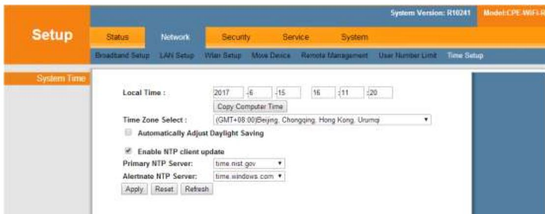
Set the time of the device, you can manually set the time or synchronize the network time.
