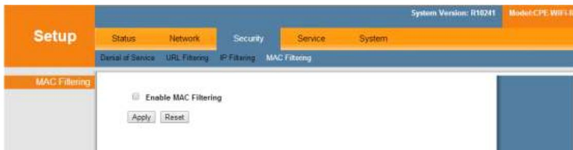
The filter is closed by default, and if you need to enable it, tick in front of the corresponding pattern and click <Apply>.
